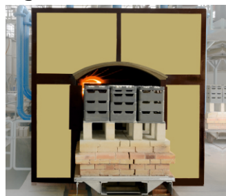
Micro processor controlled high temp. gas fired tunnel Kiln
